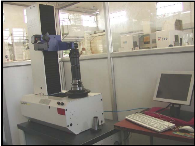
Newly Installed Tool Presetter
