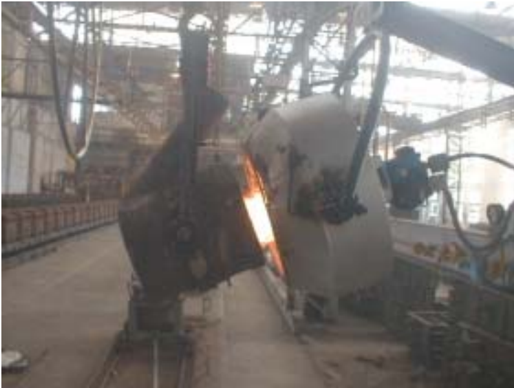
LPG based ladle- preheating system
