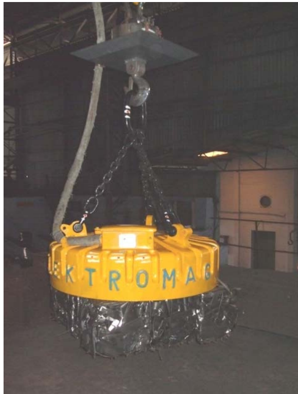
Newly Installed Magnetic Lifter
